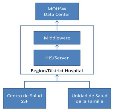
Figure 4-1. Architecture of the proposed system
