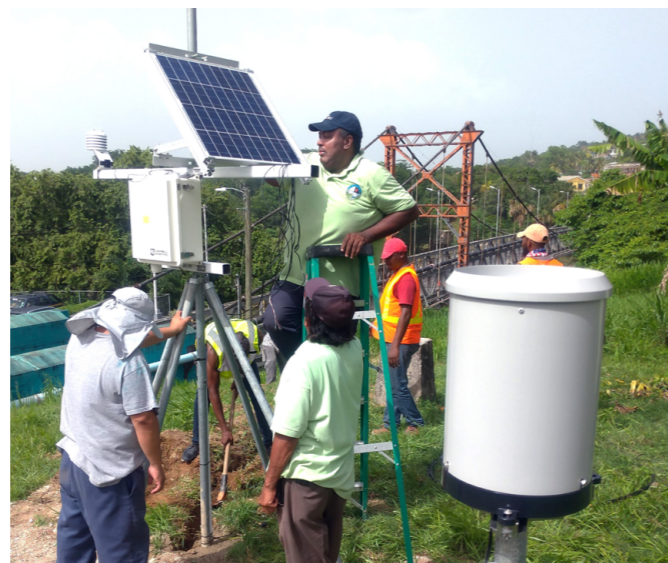
The project was able to provide 3 hours for the residents of San Ignacio to evacuate the city through a flood early warning system and IoT monitoring equipment, which provided advance warning of the flooding area and time.
