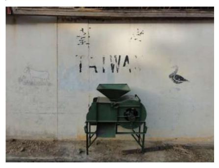
Figure 9. Rice milling equipment at a village milling station
