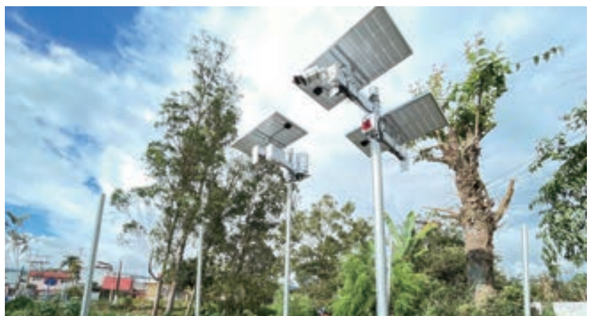
This IoT automated observation station monitors the hydrological situation in Guatemala.
