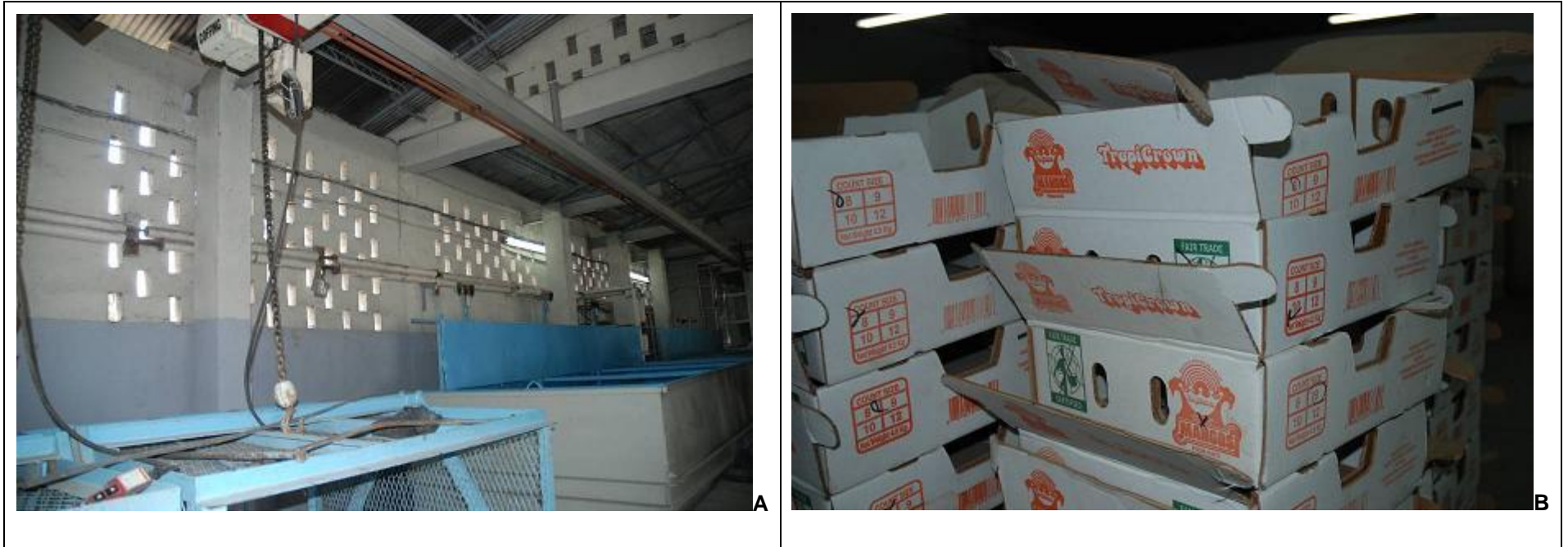
圖 4. 海地太子港芒果出口商 Perry Family Import-Export S.A. 包裝廠檢疫芒果溫湯處理設施(A)與包裝盒(B)。 Figure 4. The hot water treatment quarantine facility (A) and the corrugated boxes utilized for mango export (B) in the packinghouse of Perry Family Import-Export S.A. at Port au Prince, Haiti.
